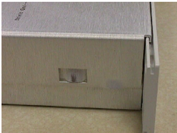
Figure 4. Front Corner of the E1529A Showing Drip Edges
